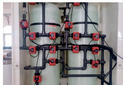
○ 电镀液重金属提取设备 Heavy metal extraction equipment for electroplating solution
